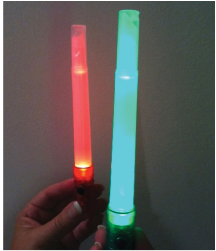
Figure 5: Press Lites separated sufficiently on the z-axis to generate physiological diplopia of the light not being fixated.
