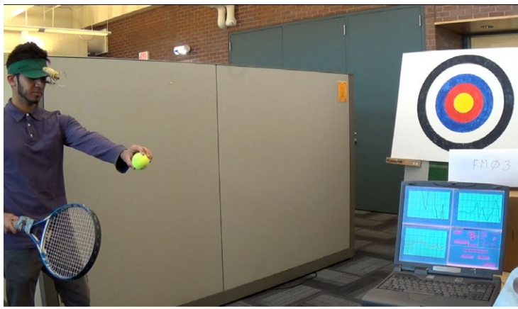
Figure 3: Experimental setup showing subject in preparation for a groundstroke to attempt to hit the center of the multi-ring bull's-eye target. The subject wore a visor with sensors for eye and head movements, while a sensor secured on the racquet handle was used to record racquet motions. In the lower-right foreground is the monitor showing the instantaneous traces of eye, head, and racquet motions as a function of time
